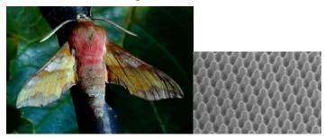
Motheye structures has been at the center of focus for researchers for its high anti reflective properties with low weave length dependency. The structures are a result of applying bio mimic technology to imitate a moth's eye.
